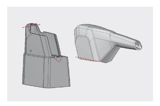
**Step 1** – Remove the handbrake plastics. This is done by pushing the plastic tab on the underside of the handbrake lever. This will allow the plastics the separate.
